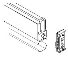
WIND BLOCK: Front bar Interlock device to be used on 100 and 130 Screeny GPZ guide, GPZ I and Gpz Unica. In wind, front bar stays locked in the low position and fabric is steadily tightened when the awning is opened completely.
