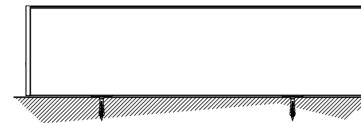
Guida a parete - Wall guide - Coulisse façade - Wandführung B-B
