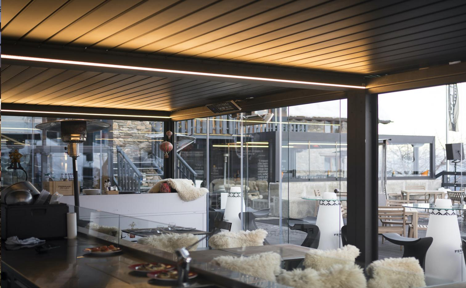
KE Isola 2 and KEDRY Plus have the LED Strip Lights option on the projection dimension of the pergola. These low voltage lights are installed inside the channel on the gutter and are dimmable by remote control. Dimmable LED strips are also available for the width dimension as well.
